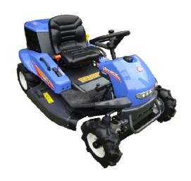
The SRA 800 and 950F are ride-on brush cutters capable of cutting grass and thick vegetation right up to saplings. Their low height aids stability when used on slopes. Both machines are powered by Kawasaki electric start petrol engines – 16 hp & 24 hp respectively and have hydrostatic drive – 4WD for the SRA950F. Cutting widths are 80 cm or 95 cm.
