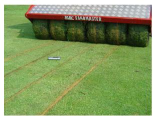
The combination of the Ground Breaker and Sandmaster working in tandem can produce a matrix of sand slits at 26cm centres with virtually no surface disturbance.
